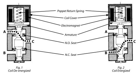
**The De-energized Position** With the valve in a de-energized position and pressure applied to Port B, the valve operates as a 3-way, 2-position, normally closed valve. In this position a flow pattern from Port A to Port C is established (figure 1). Pressure can be applied to either port. The forces affecting the poppet are on the normally closed seat resulting from the poppet return spring.
